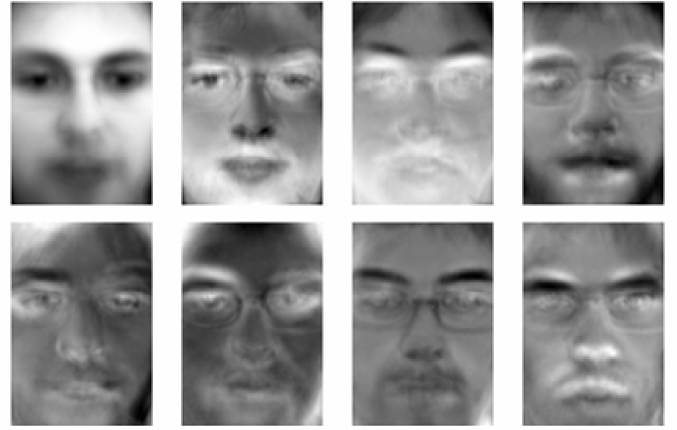
Fig. 6. Upper left corner: mean face image from the whole face database. From left to right, the whole database eigenfaces associated with the 7th largest eigenvalues are shown in decreasing order.
